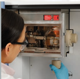
1) Simply remove radial torch and interface
