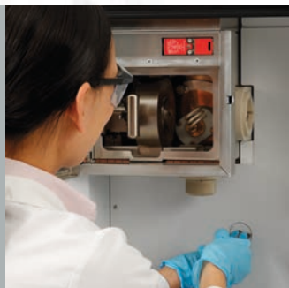
2) Rotate load coil into desired horizontal orientation
