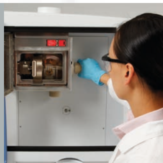
3) Install axial torch and interface
